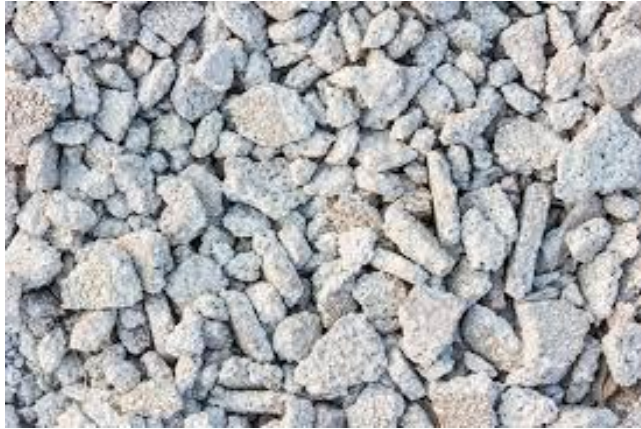
Figure 2: Recycled Concrete Aggregates (RCA)
