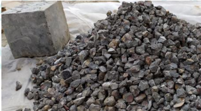
Figure 2: Recycled Concrete Aggregates (RCA)
